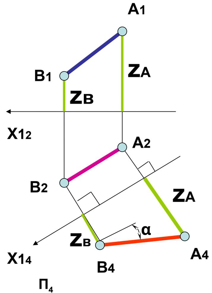
$$\left\{ \begin{array}{l} \pi_4 \perp \pi_2 \\ \pi_4 \parallel AB \end{array} \right. \quad X_{14} \parallel A_2 B_2$$
