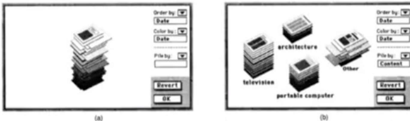
Figure 6. Visualizing a pile's contents . The pile shown is within a 'visualizing environment' that allows the user to select and visualize several criteria. Criteria can be mapped to the pile's order, the color of the items within the pile, or the way a pile is broken into sub-piles. In (a) the pile is both ordered and colored by date. In (b) the user chose to 'pile by' content. Therefore, the system separated the original pile into four content-based piles. Three are labeled with specific terms suggested by the system (e.g. "architecture"), appear neat and are now scripted to maintain similar content. The remaining disheveled pile, "other," contains items which did not fit into any of the other three piles.
